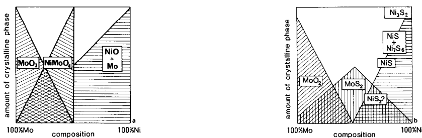
FIG. 1. Schematic composition diagrams of the crystalline components found by X-ray and electron diffraction of the binary Ni-Mo system: (a) oxides; (b) sulfides used as catalysts.
