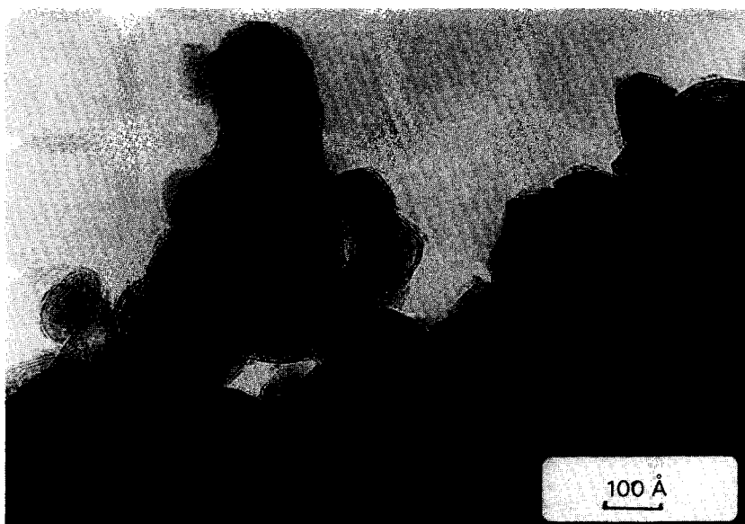
FIG. 11. Electron micrograph of sulfided sample B showing how the small crystals of NiMoO 4 , C in Fig. 4, are converted to expose a skin of MoS 2 , 2 to 10 layers thick.
